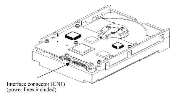
Figure 4.9 Connector location
